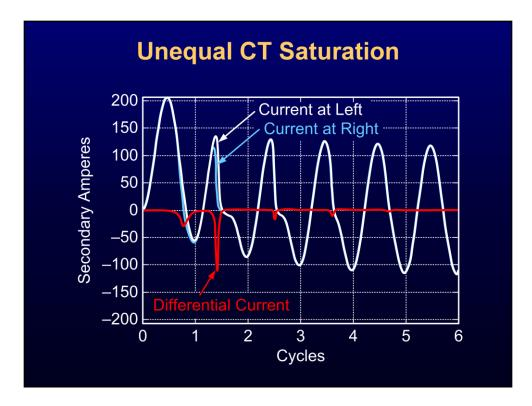
The slide shows the results of a simulation produced SEL software. Even though both CTs in this case are similar, slight differences in the CT characteristics create a differential current during saturation.
