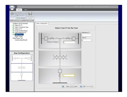
To conduct tests in the Commissioning Assistant software, assign any two windings to the test. One winding serves as the reference CT and the other as the test CT input. The software then reads the current magnitudes and angles from the relay and compares them with the compensation settings and CT ratios used in the relay.
