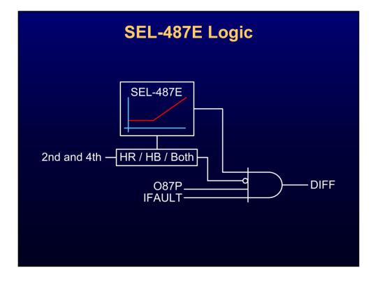
The SEL-487E has a single-slope differential element that uses internal versus external fault detection logic to switch the slope of the differential restraint to a higher (more secure) level when external faults are detected.
