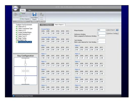
This slide demonstrates the capabilities of the Commissioning Assistant software. The first step is to define the transformer connections and type. The Commissioning Assistant software offers the choice of IEC or IEEE transformer representations.
