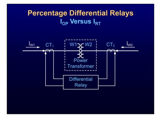
This slide shows the differential scheme applied to the protection of a power transformer.
