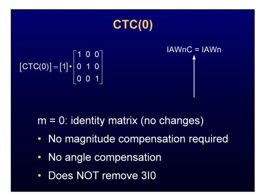
This internal relay equation represents m = 0. The notes on this slide and the following slides all show the equations for the respective matrix shown on the slide.
