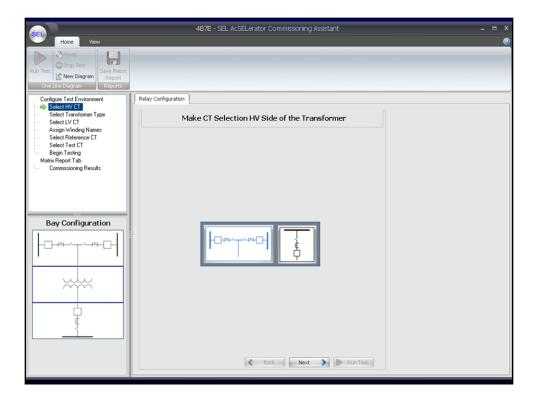
Using the SEL ACSELERATOR QuickSet<sup>®</sup> SEL-5030 Software Commissioning Assistant is easy. Simply select the Commissioning Assistant tab, and start by defining the one-line diagram of the transformer and interconnecting breakers.
