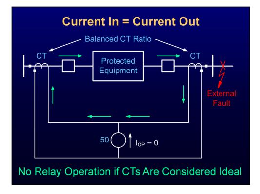
The slide shows the behavior of the simplest differential scheme (using an instantaneous overcurrent relay) during an external fault. If the CTs are considered ideal and identical, the primary and secondary currents at both sides of the protected equipment are equal. There is no operation (differential) current.
