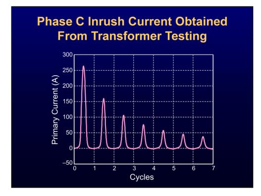
This slide shows a typical example of inrush current.
