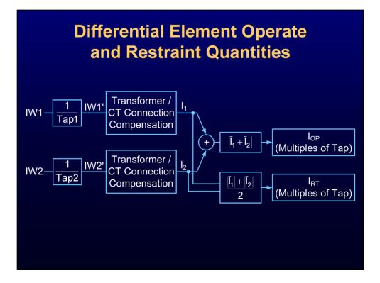
After tap, phase, and zero-sequence compensation, the differential elements develop  $I_{OP}$  as the phasor addition of the currents and  $I_{RT}$  as the average of the magnitudes of the currents.
