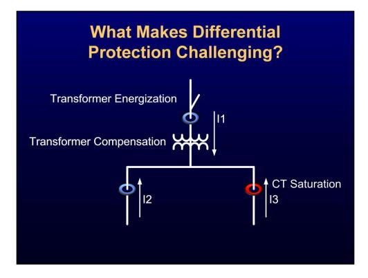
The main challenges to any differential protection scheme come when, under normal operating conditions, the current into the differential zone may not equal the current leaving the zone. This basic protection presentation examines the following differential protection challenges:
