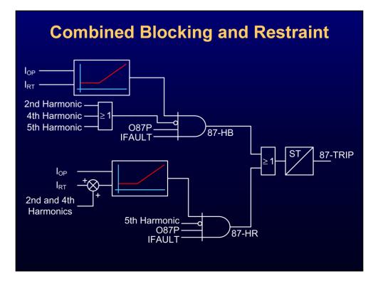
The SEL-487E and SEL-787 allow harmonic blocking and restraint to be combined. This provides the speed of harmonic blocking for inrush conditions that have consistently high levels of second and fourth harmonics and the security of harmonic restraint for inrush conditions that have lower levels of harmonics or erratic harmonic content.
