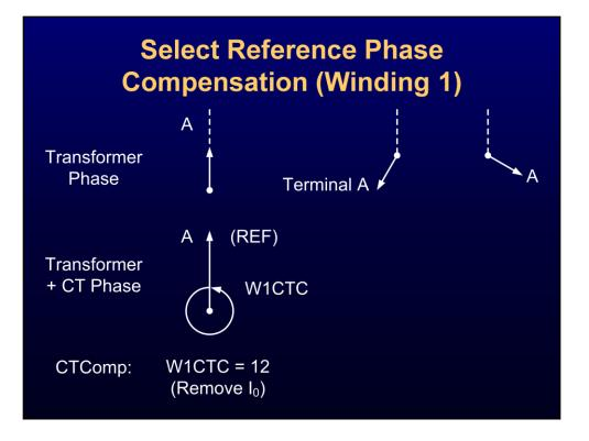
The transformer phase positions from the previous slide are shown at the top of this slide for reference. The next step is to adjust the Phase A positions for the indicated CT connections. The CTs are connected in wye for the first two windings and in a DAC, or 30-degree lagging delta, for the third winding.
