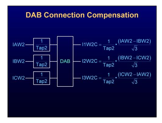
With DAB compensation, the currents are first tap adjusted and then combined mathematically as they would be in a delta  $\bar{I}_A - \bar{I}_B$  CT connection. The resultant phasors are divided by the  $\sqrt{3}$  factor to eliminate the increase in magnitude caused by the delta phasor subtraction.
