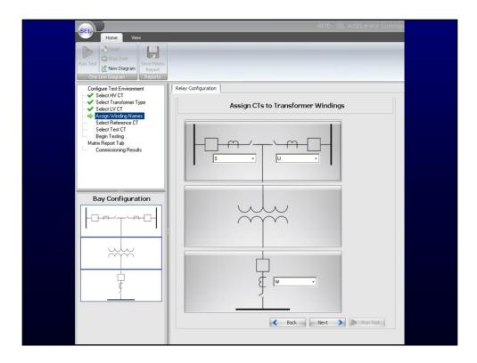
Once the one-line diagram is complete, select the windings that will be used as differential element inputs to the relay.
