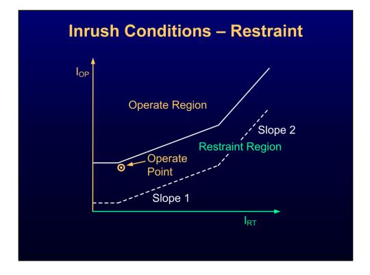
Harmonic restraint raises the transformer characteristic by a constant value c, which is the sum of the second and fourth harmonics. This happens independently in each of the three differential elements. For example, Phase A is unaffected by the harmonic content of Phase B and Phase C.
