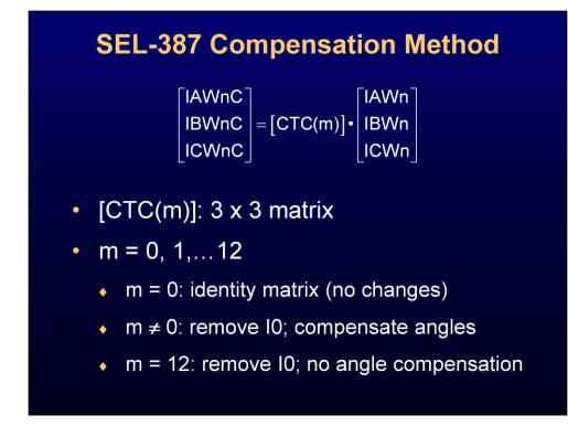
Some transformer and CT connections require more than 30 degrees of phase shift. The SEL-387 expands on the concept used in the SEL-587 by using settings like the hours on a clock that provide complete 360 degrees of phase shift in 30-degree increments.
