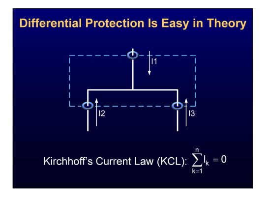
In theory, differential protection is a straightforward undertaking. Following Kirchhoff's Current Law (KCL), the sum of all currents at any node in a circuit must equal zero. Current in must equal current out.
