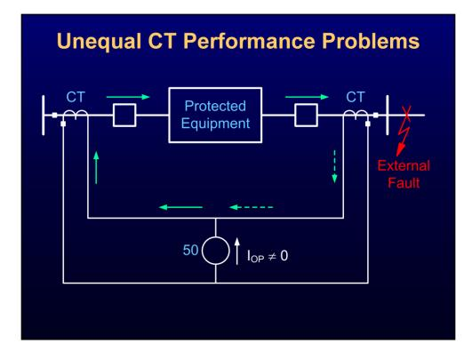
All differential protection must deal with the challenge of being secure for large through faults. During a severe external fault, a CT may saturate and supply less than its ratio current. In this case, the currents do not completely cancel, and a false differential current results. When high currents are present, use some measure of through current to desensitize the relay.
