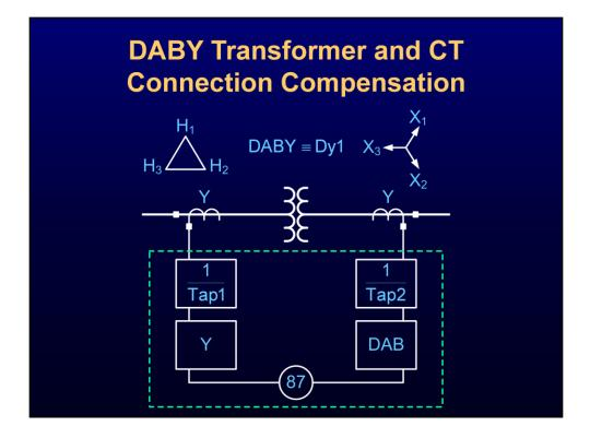
This slide shows a delta-wye transformer with 30-degree lag (ABC phase sequence).
