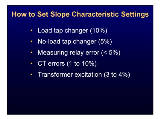
Several factors typically go into selecting the Slope 1 percentage slope setting, including the following:
