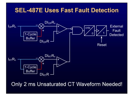
As shown on the previous slide, the SEL-487E only operates with one slope active at a particular instant in time (this allows for greater sensitivity during internal faults and greater restraint during external faults). To accomplish this task, the SEL-487E has an external fault detector that is capable of detecting the presence of an external fault within 2 milliseconds.
