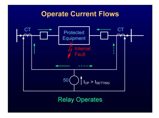
For an internal fault, the primary currents allow the secondary currents to produce a differential current through the overcurrent relay. If this differential (operation) current is larger that the relay pickup, then the relay trips both circuit breakers instantaneously.
