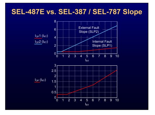
While the traditional dual-slope characteristic has been shown to be very reliable for preventing operation during external faults with CT saturation, the single-slope characteristic has been designed to provide high sensitivity for internal faults and rapid transition to the higher slope during external faults. Testing has shown that the adaptive differential element is better at handling evolving faults and external faults with very severe CT saturation.
