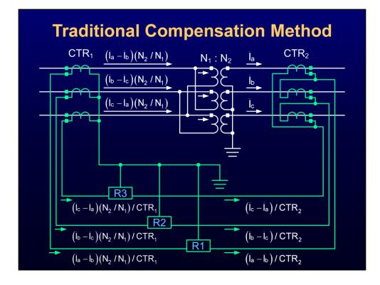
When traditional electromechanical relays are used, the CTs must be properly connected, as shown by the figure on the slide (DAC power transformer).
