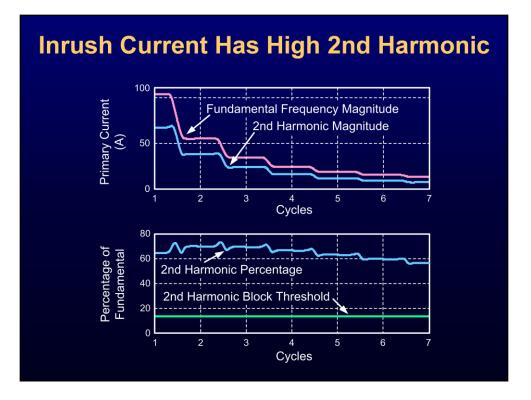
Analysis indicates a significant amount of second harmonic in the waveform shown on the slide.
