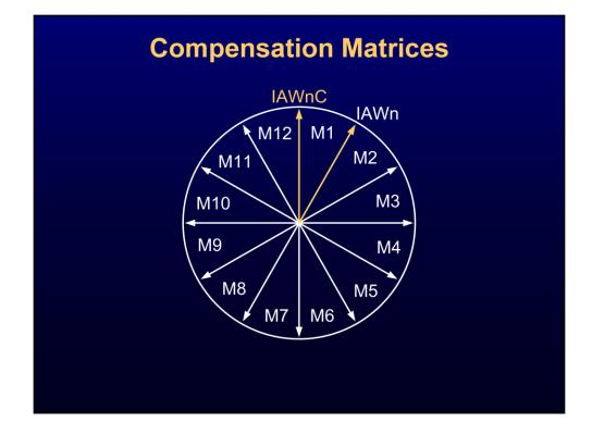
The next several slides describe the twelve compensation matrices used in the SEL transformer differential family of relays.
