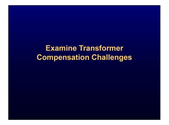
Another challenge in differential protection occurs when a transformer is placed within the differential protection zone. The transformer induces differences in current magnitudes within the zone due to the transformation ratio. Differences in transformer winding configurations (delta, wye, and so on) also induce phase angle differences in the current vectors that must be compensated for.
