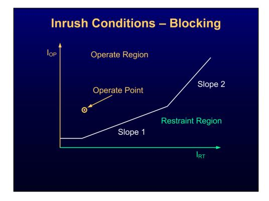
Consider relay operation for the harmonic blocking selection. The operating point  $(I_1 - I_2)$  is in the trip region, and the transformer should now trip. However, before the trip command is issued, the harmonic conditions are evaluated. If the percentage of harmonics exceeds the setting, relay operation is blocked.
