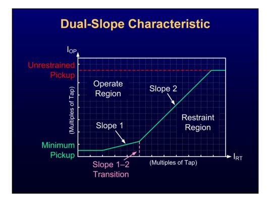
The figure on the slide is a graph of a dual-slope percentage restraint characteristic.
