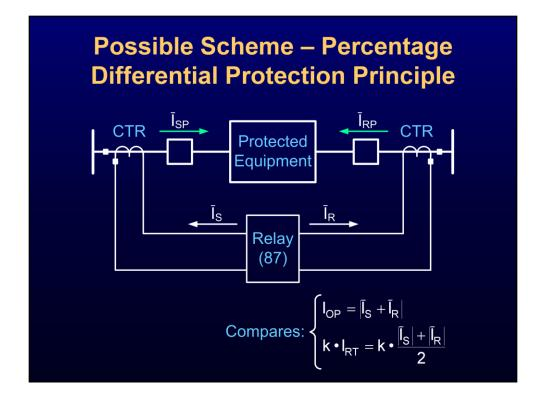
A common variation on the differential concept is the percentage restraint differential relay. The differential elements compare an operate quantity with a restraint quantity.
