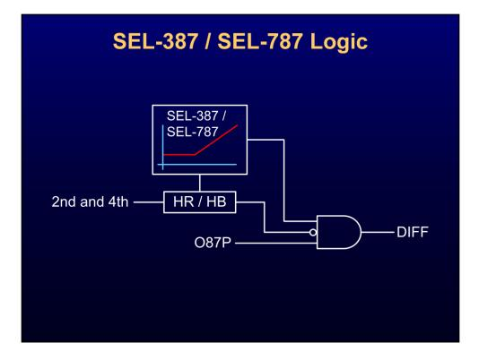
Recent additions to the SEL differential protection relay lineup include the SEL-487E and SEL-787 Transformer Protection Relays. The SEL-787 provides a two-slope method that is also used in the SEL-387 Current Differential and Overcurrent Relays and the SEL-587 Current Differential Relays.
