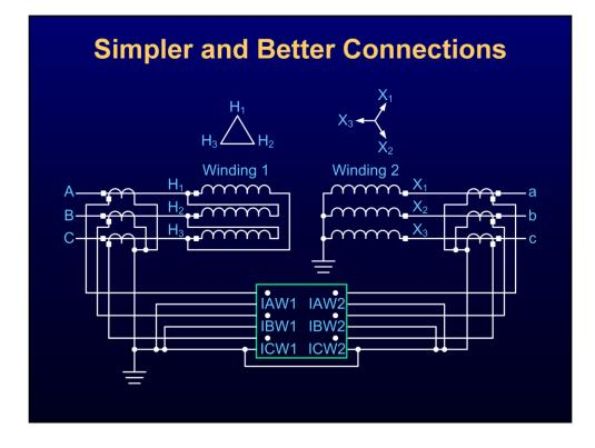
With numerical relays, it is possible to connect the CTs in wye and let the relay calculate the delta compensation. This method has the following advantages:
